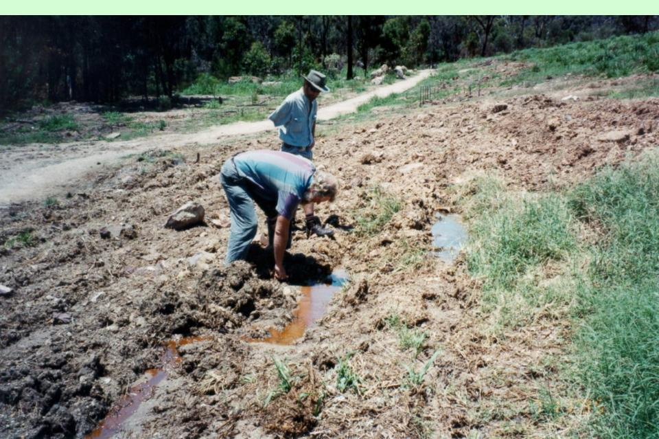
This leachate runoff is highly contaminated with Chromium, Cadmium, Copper, Lead and Zinc. It will eventually run into a nearby creek
